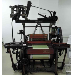
〈Fig. 26〉 Dobby Machine Tokyo University of Agriculture and Technology collection (Photographed by author, 2016)
