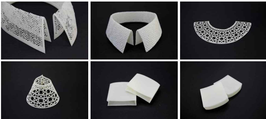
<Fig. 13> TPU Material, Color Printed by SLS Method, Cuff and Pocket
