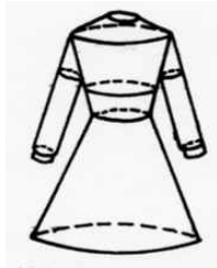
<Fig. 2> Convert to 3D geometry: cone, inverted cone, cylinder, ring (Davis, 1996, p. 101)
