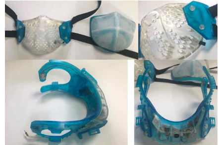
〈Fig. 25〉 The printed and assembled mask platform and Bluetooth systems
